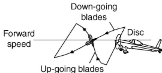
*As the tail of aircraft is down, the axis of rotation is inclined. The down-going blade produces greater thrust as it is at higher angle of attack than the up-going blade. This causes asymmetric loading and aircraft making the aircraft tending to yaw.*
